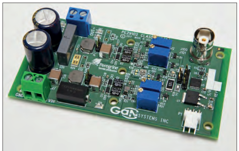
Image 1. The 100 V GaN E-HEMT FB EVB (GS61004B-EVBCD) optimized for Class D amplifiers.
